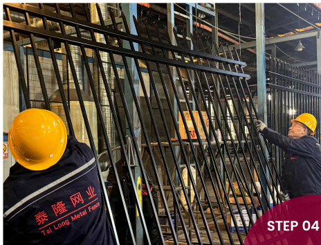
Steel Fence Panel Powder Coating
