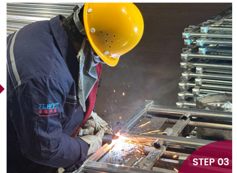
Steel Picket Fence Panel Welding
