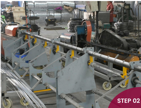
Teel Wire Straightening
