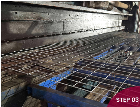
Wire Mesh Welding
