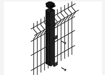
Metal Clamp Connection
