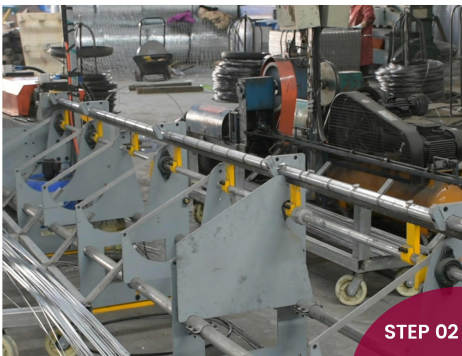
Steel Wire Straightening And Cutting
