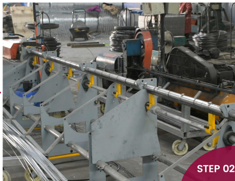
Steel Wire Straightening And Cutting
