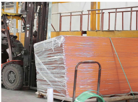
EDGE PROTECTION BARRIER DELIVERY
