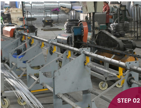
Teel Wire Straightening And Cutting
