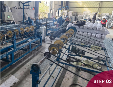
Chain Link Mesh Weaving
