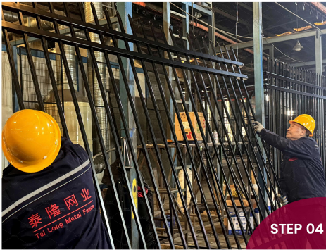
Steel Fence Panel Powder Coating
