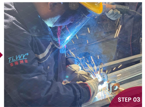
Steel Picket Fence Panel Welding
